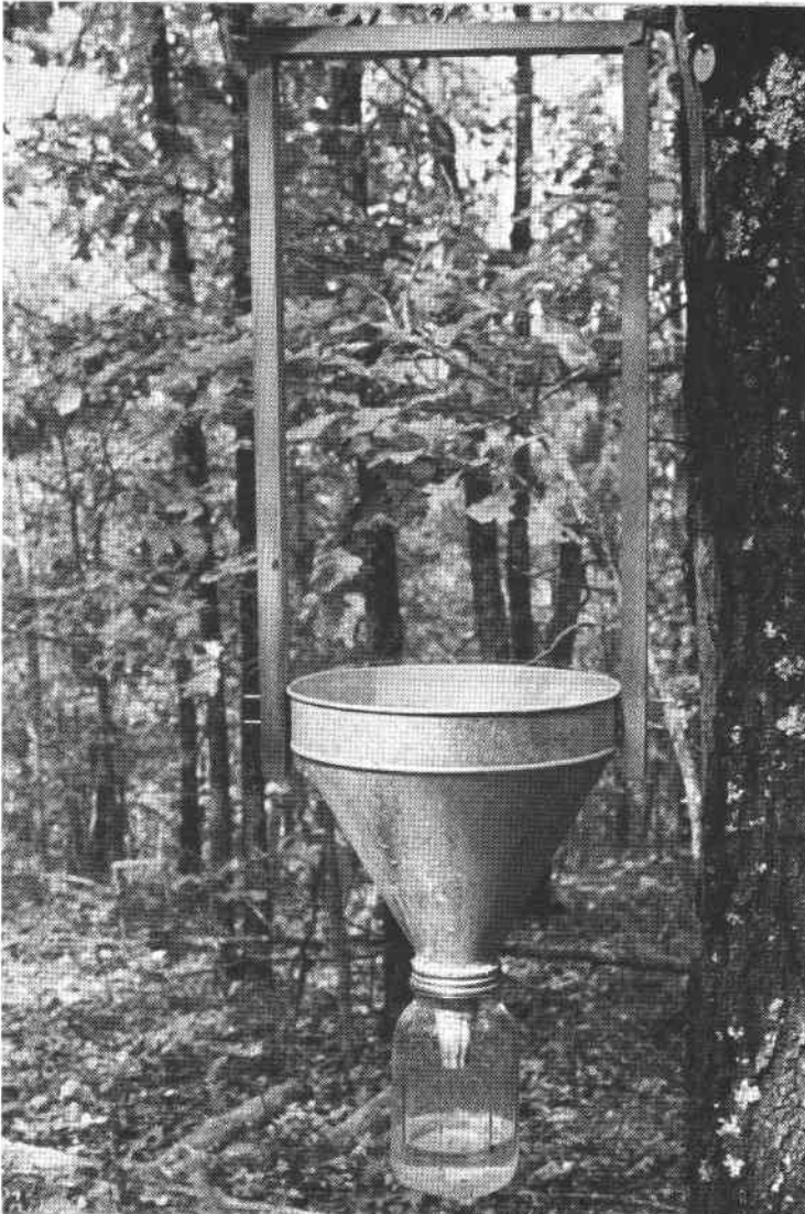
FIG. 1. Window flight trap used to trap scolytids.
